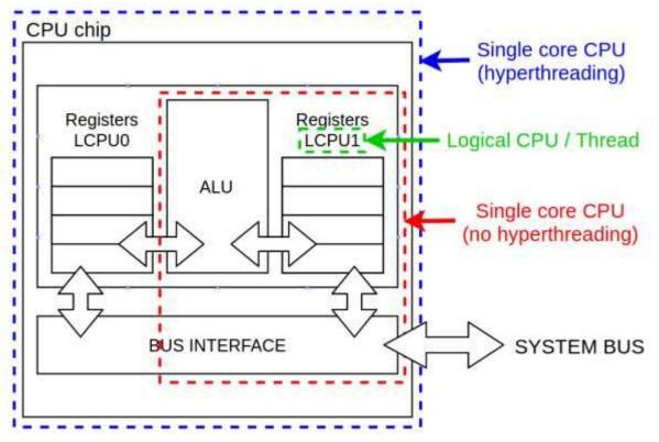
Single core hyperthreading CPU (2 logical CPU's / threads)
